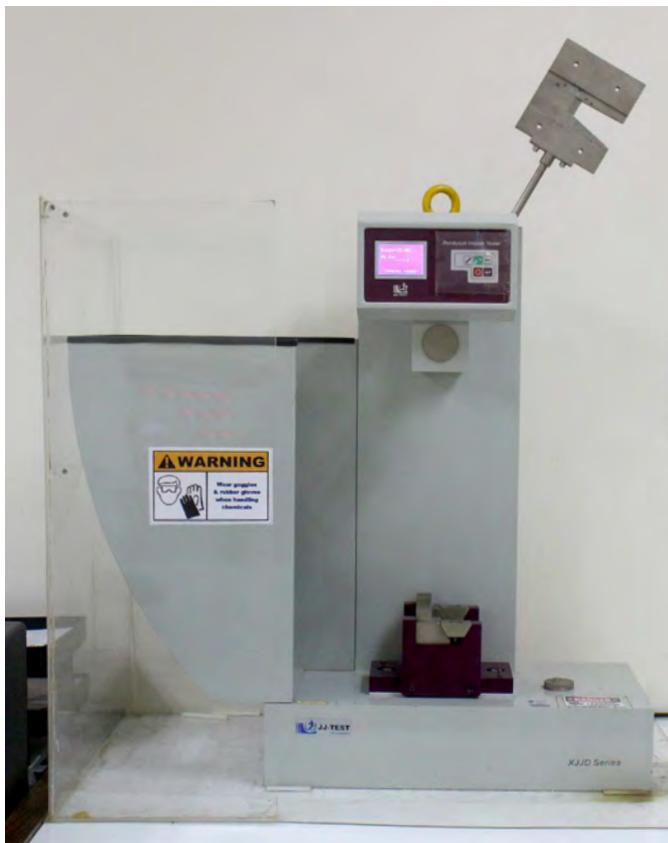
Fig. 7: VESBO® Pendulum-type Impact Test Equipment
