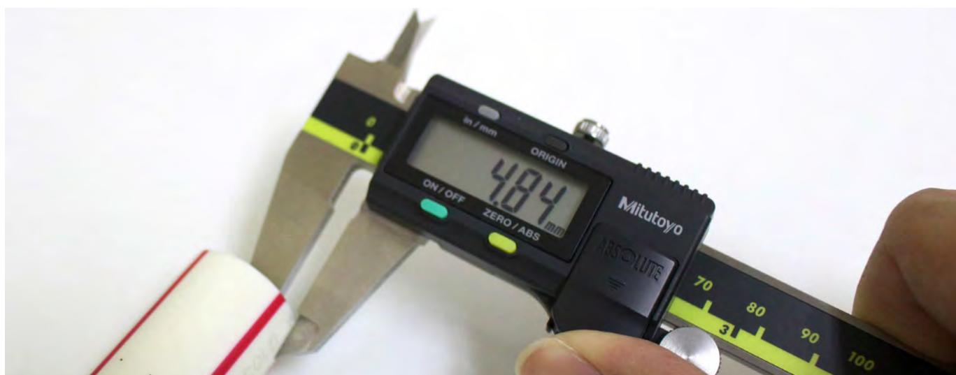
Fig. 6: VESBO® Dimensional Test Caliper
