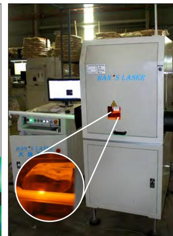
Fig. 15: Code Marking Machine
