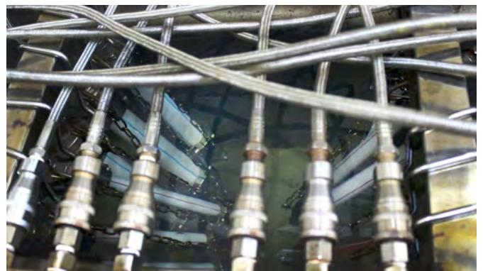
Fig. 8: VESBO® Creep Test Water Bath
